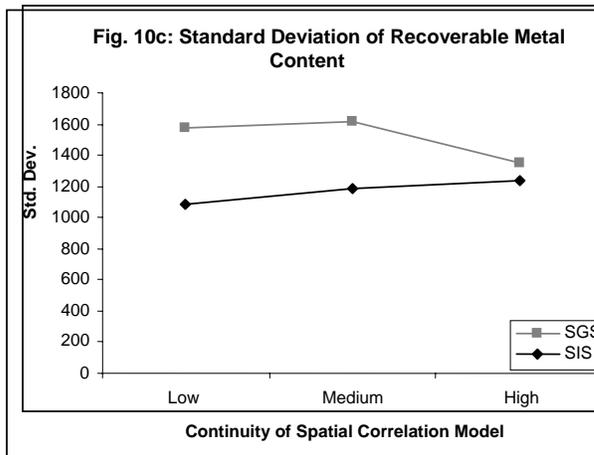
**Figures 10a to 10c:** Comparison of the uncertainty measure (standard deviation) of different transfer functions applied to SGS and SIS results in the SMU scale.
