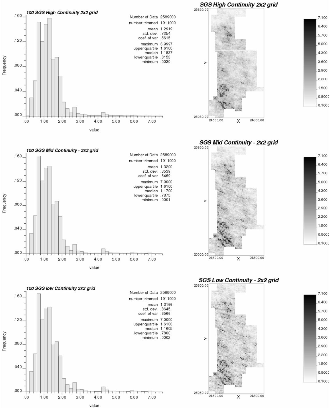
**Figure 3.** Left: Histograms of all simulated values by SGS with high (top), middle and low (bottom) spatial continuity variogram models. Right: sample realizations.
