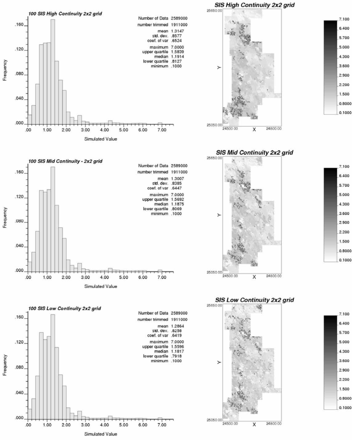
**Figure 4.** Left: Histograms of all short scale simulated values by SGS with high (top), middle and low (bottom) spatial continuity variogram models. Right: sample realizations.
