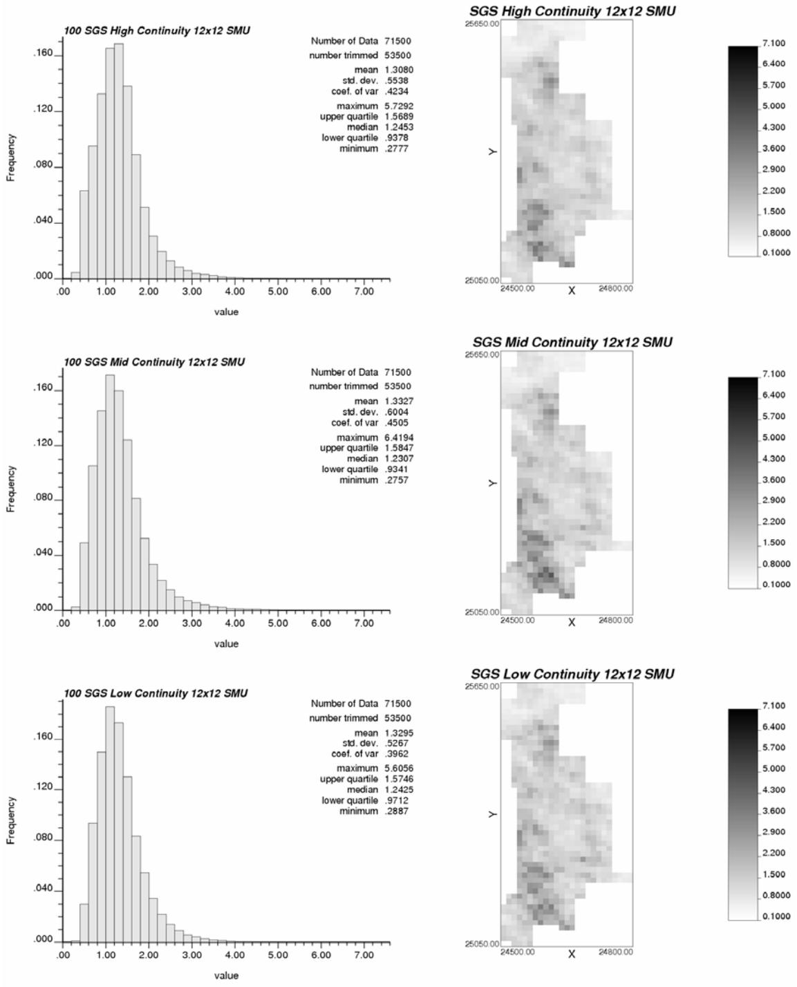
**Figure 5.** Left: Histograms of SGS results averaged in a 12m x 12m SMU scale corresponding to high (top), middle and low (bottom) spatial continuity variogram models. Right: Sample Realizations.
