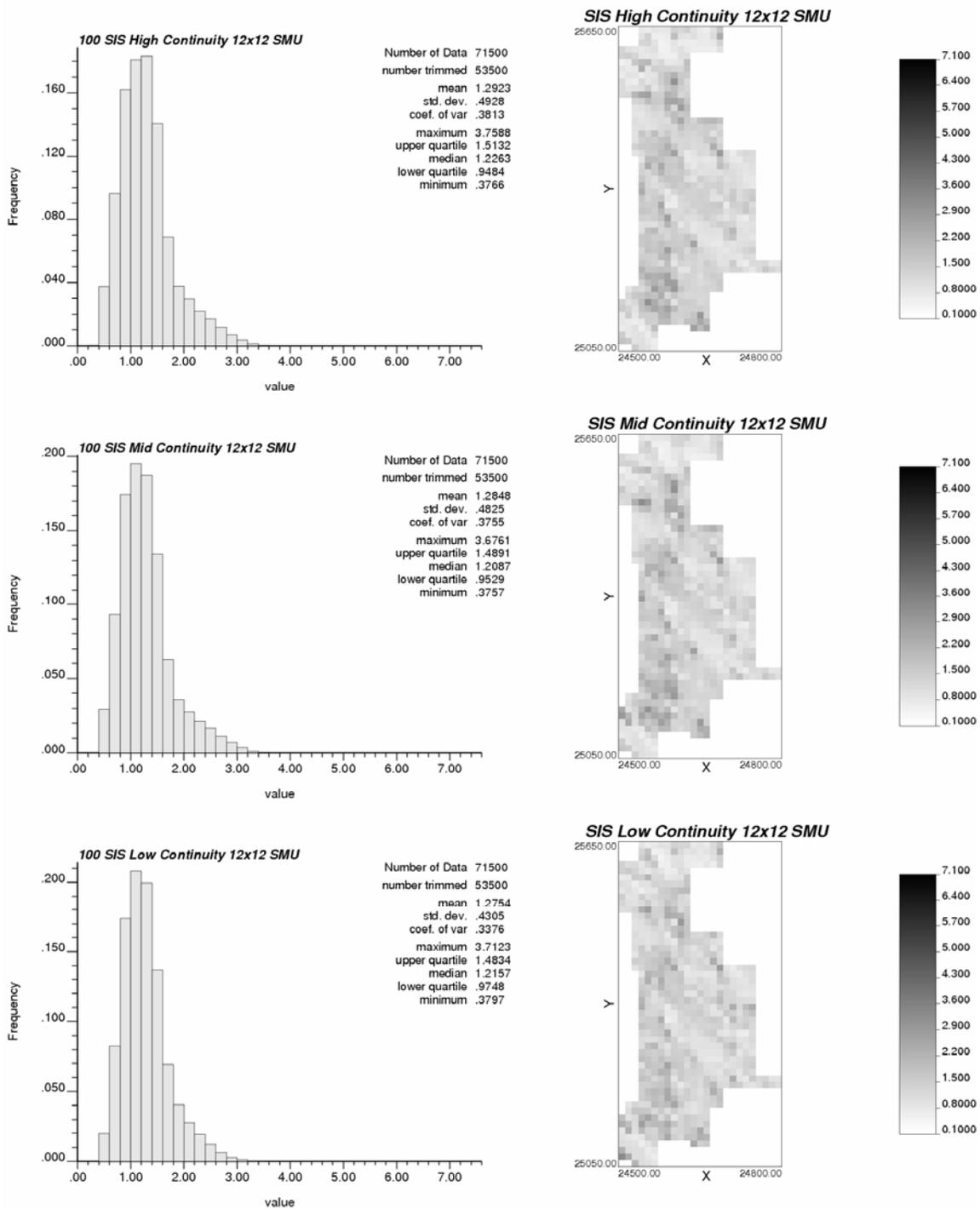
**Figure 6.** Left: Histograms of SIS results averaged in a 12m x 12m SMU scale corresponding to high (top), middle and low (bottom) spatial continuity variogram models. Right: Sample Realizations.
