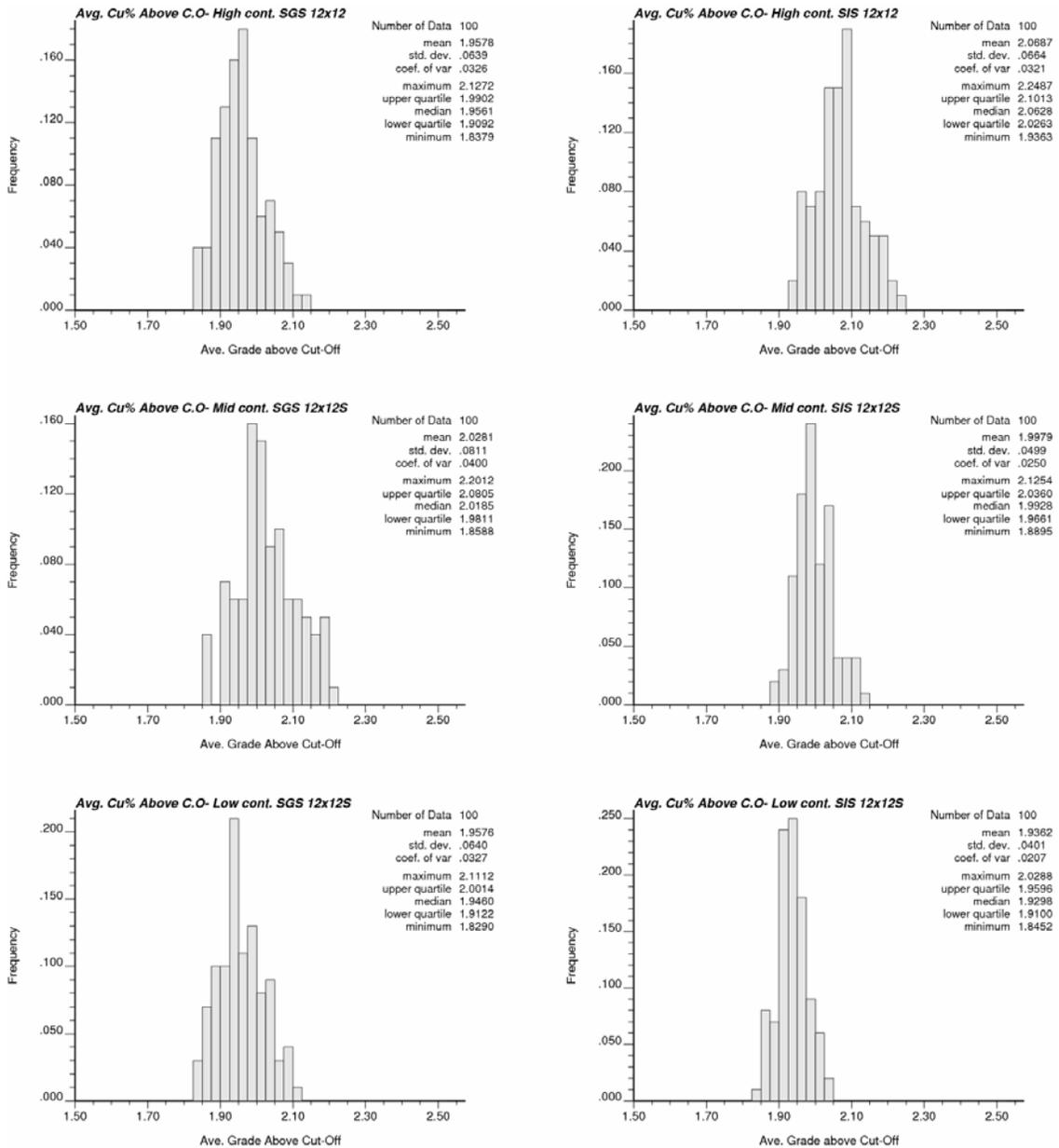
**Figure 8:** Histograms of the average grade above cut-off for 100 SGS (left) and 100 SIS (right) realization using different spatial continuity models.
