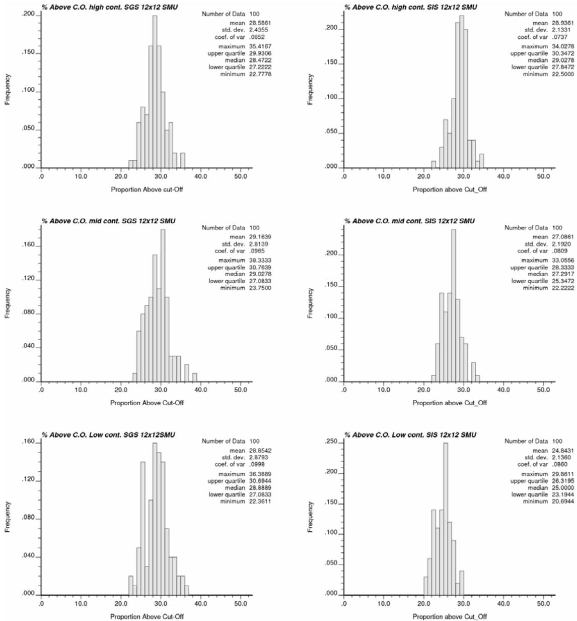
**Figure 7:** Histograms of the proportion of recoverable Tonnage for 100 SGS (left) and 100 SIS (right) realization using different spatial continuity models.
